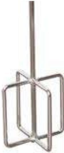
With mixing, the goal is to use the mortar as dry as possible. Excess water leads to shrinkage as the material dries out. Mortar that is too wet must be compacted in lifts (layers) while it is drying to ensure proper adhesion and carbonation. Using the mortar with a very stiff consistency lessens the need to compress it in the wall, makes it less messy to work with, and keeps wall faces cleaner.
